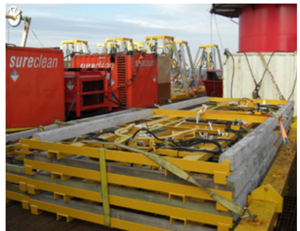
NORTH SEA Retrosled aboard a vessel bound to retrofit the Forties infield flowlines
