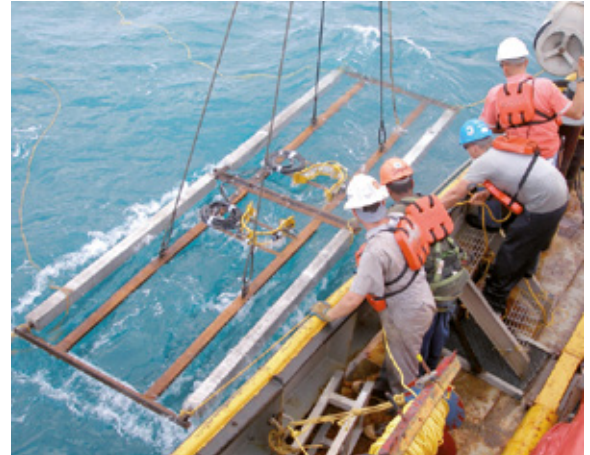
GULF OF MEXICO Retrosled with two clamps being overboarded
