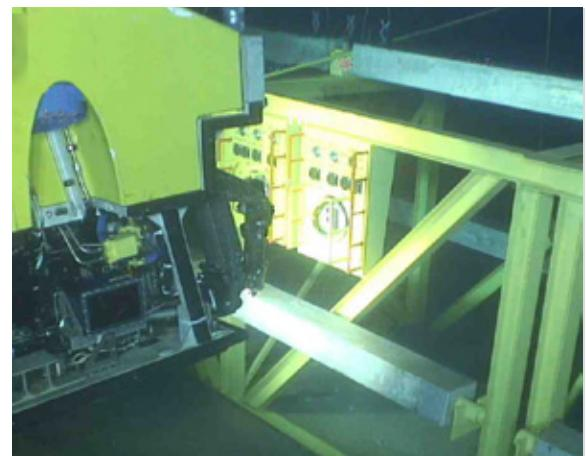
**SUNSTATION MOUNTED ON AN ANODE SLED**
