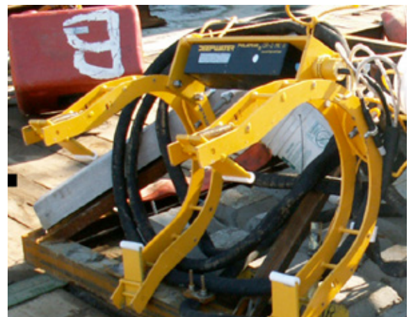
RETROFITS DR-2 to be retrofitted to a subsea pipeline attached to two RetroClamps.
