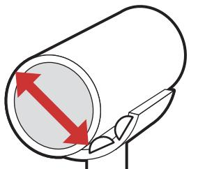
Provide the outer diameter of the pipe (or the nominal diameter) so we can determine the correct radius for the inside of the I-Rod Clip.
