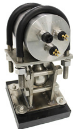
REAR VIEW OF DEEP C METER 3000 AD DISPLAY Whips attach here for ROV II, EFG probe and digital data stream.
