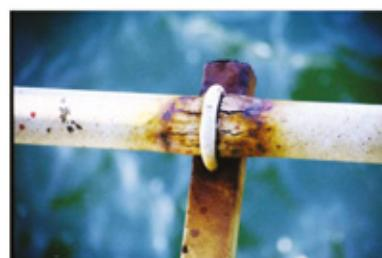
Topside crevice with the destruction in the water trap. Corrosion process will deteriorate the metal to the electrode.
