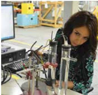
Deepwater's corrosion laboratory covers 3,000 square feet and boasts a fully-pressurized test chamber, potentiostats, 6,500 gallons of test tanks, and anode testing facilities.
