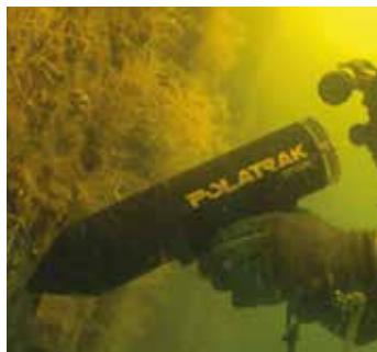
Deepwater has been conducting offshore surveys for three decades. The diver at right is using Deepwater's Polatrak® CP Gun to take cathodic protection readings.
