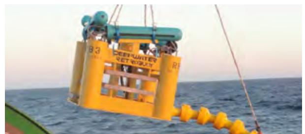
FIG. 2: 950-AMPERE ICCP BUOYANT ANODE SKID This is one of eight that were installed
