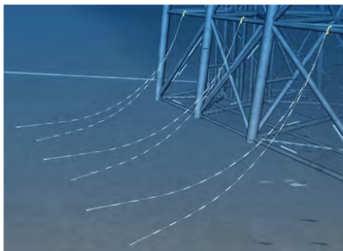
FIG. 14: LINK ANODES SHOWN IN "SKIRT LINK DEPLOYMENT" Installed using a shallow air six-man dive crew
