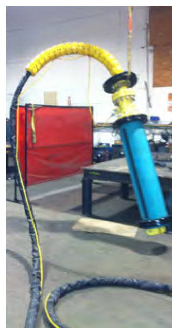
FIG. 9: SUSPENDED ANODE MODULE Uses balcony-mounted recovery
