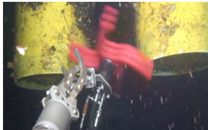
FIG. 7: ROV FLEXICLEAN SYSTEM Reduces cleaning time for subsea installations
