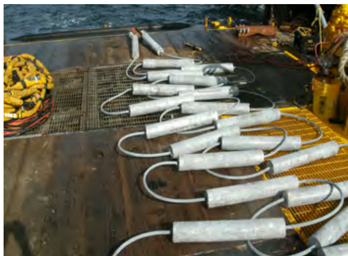
FIG. 14: LINK ANODES SHOWN IN "SKIRT LINK DEPLOYMENT" Installed using a shallow air six-man dive crew
