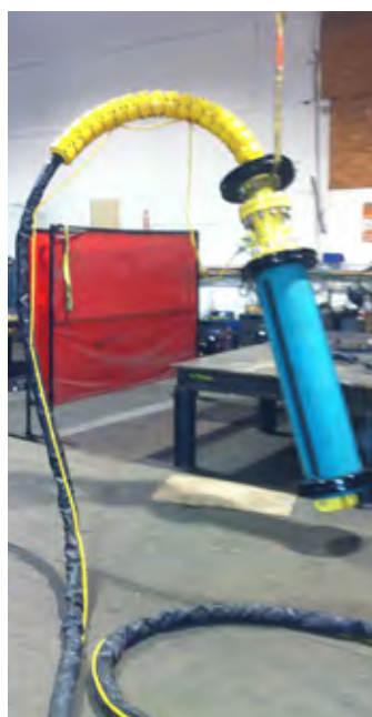
FIG. 9: SUSPENDED ANODE MODULE Uses balcony-mounted recovery
