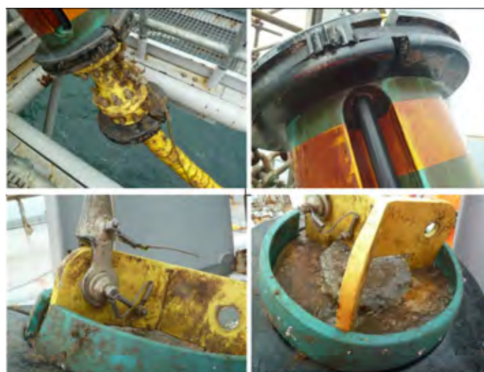
FIG. 12: HOW IT HOLDS UP Condition of the module after 18 months in service
