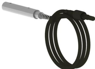
**3. Remote Electrode Adapter Cable** – This cable has the appropriate connector for the TMS electrode on one end and the remote reel on the other and is used to adapt the remote electrode of choice to the topside or TMS MUX. Choose the appropriate connector for your application and cut the cable to the desired length.
