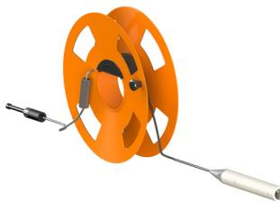
**2. Tether Management System (TMS) Mounted Probe** – Twin electrode CP probe suitable for remote variance measurements when attached to the tether management system (TMS) of an ROV. The use of this probe requires copper conductors from the ROV to the TMS.
