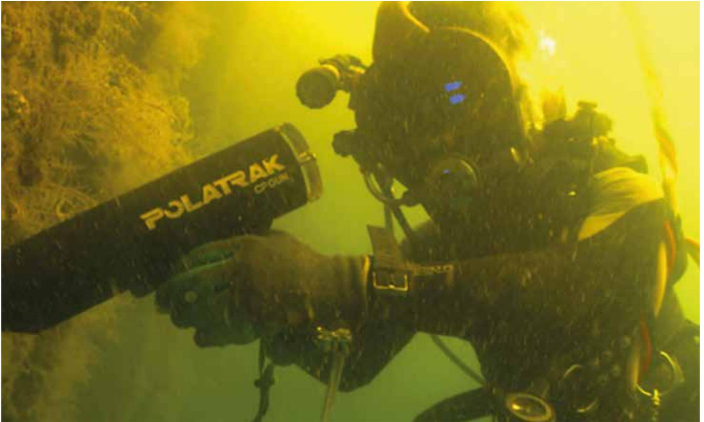
Polatrak probes are designed with dual reference electrodes for accuracy and interchangeable spare parts for service in the field. Unlike other cathodic-protection testing equipment, all Polatrak probes are designed with dual elements. Silver chloride electrodes provide the greatest accuracy offshore, but they can also require frequent re-calibration.
