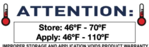
If the contractor cannot guarantee that the I-Rod Adhesive cannot be stored at the correct temperature, the surface is properly prepared, and the I-Rod Adhesive cannot be applied at the correct temperature, then we recommend bolting over the use of the adhesive.
