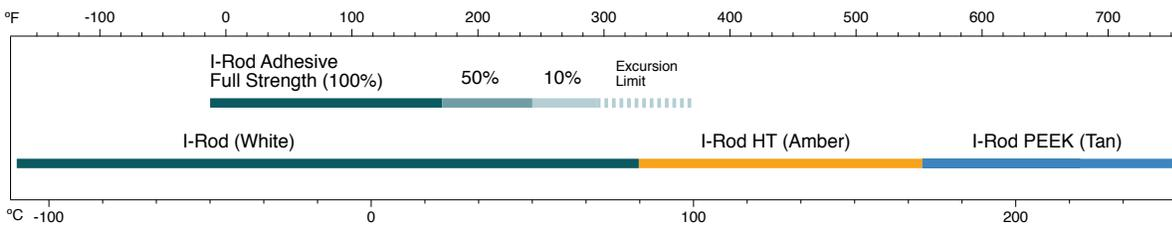
Figure 3: I-Rod strips and I-Rod Adhesive Useful Ranges
