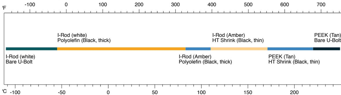
Figure 2: Recommended Nu-Bolt Configuration for a given continuous maximum temperature range.
