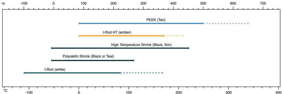
Figure 1: Temperature ranges of Nu-Bolt Materials
