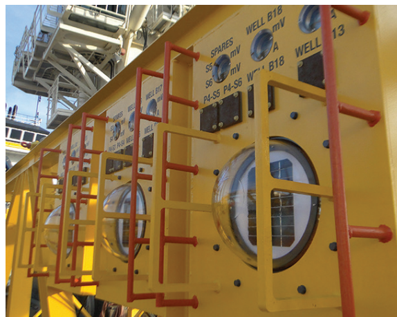
SUNSTATION™ MONITORING Each asset is monitored with a readout that's actuated by an ROV's lights.
