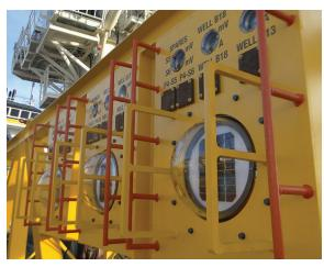
SUNSTATION™ MONITORING Each asset is monitored with a readout that's actuated by an ROV's lights.
