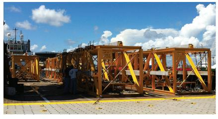
A BOATLOAD OF CATHODIC PROTECTION Four RetroPod™XL anode sleds will protect 24 PGBs in the Olympus Field.
