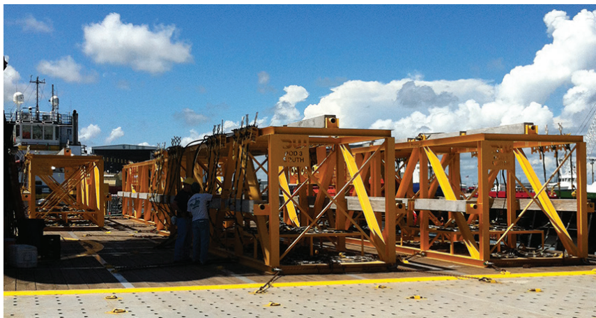
A BOATLOAD OF CATHODIC PROTECTION Four RetroPod™XL anode sleds will protect 24 PGBs in the Olympus Field.
