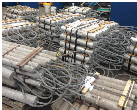
BOATLOAD OF ANODES These were the anodes used to protect all 47 steel columns of the pier.
