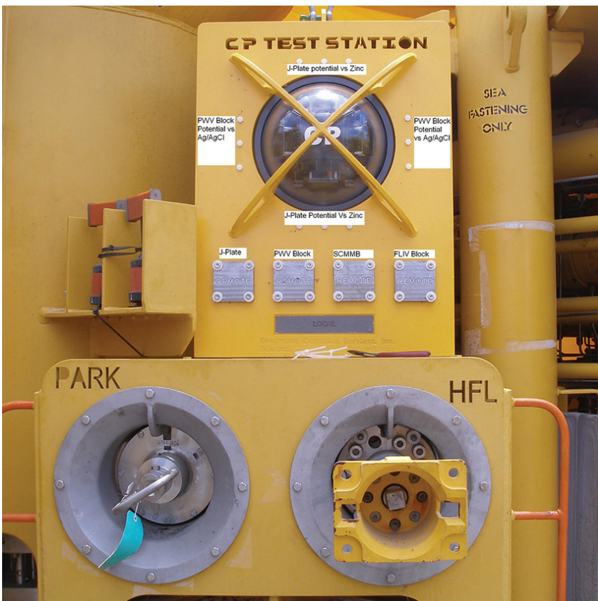
PERMANENT MONITORING STATION Completely powered by an ROV's lights, there is no battery to wear down. It can operate subsea for up to 25 years.
