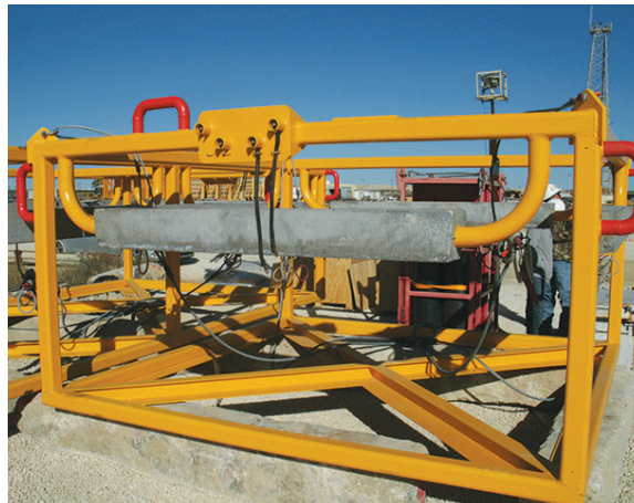
NOT-SO-TOUGH SLEDDING The anode sleds will provide flowlines with CP once they're connected..
