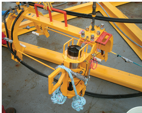
RETROREADER™ BEFORE DEPLOYMENT The reader will verify electrical connection through the flowlines' coating.
