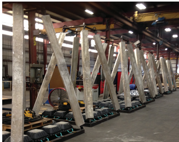
AWAITING DEPLOYMENT Seven RetroPods™ were used to cathodically protect the two structures.
