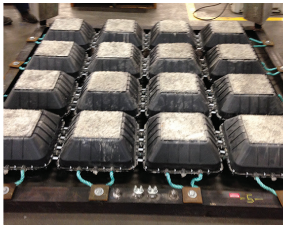
STABILITY IN STRONG CURRENTS Concrete mats were added to the base of the RetroPods™ for stability.
