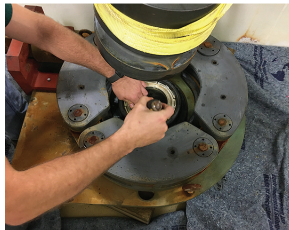
CLAMP CONNECTOR'S CATHODIC CONUNDRUM Searching for the cause and effect of CP on a subsea 725-alloy gasket.
