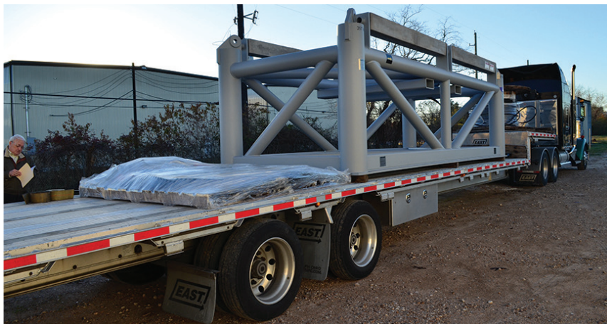
CUSTOM DESIGN In addition to our standard designs, Deepwater can build anode sleds tailored for use in special conditions.
