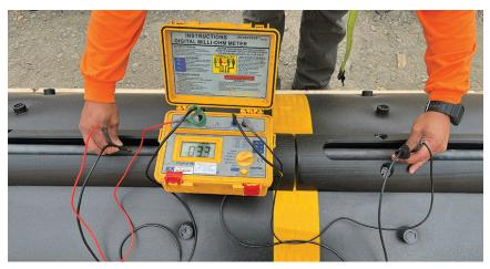
**DOUBLE-CHECKING THE ANODES**A technician tests the anodes once again before installation.
