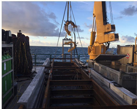
THE RETROSLEDS™ ABOUT TO VISIT THEIR NEW HOME The attached RetroClamps™ will provide the electrical connection.
