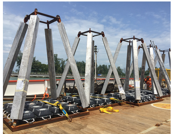
RETROPODS™ IN A ROW Lower-profile RetroSleds™ were used on the pipeline retrofit.
