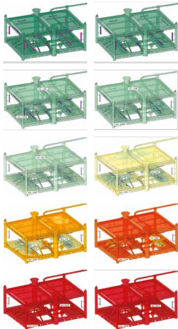
AS-BUILT ANODE OUTPUT MODEL PROGRESSION (FROM NEW TO DEPLETED) Top left shows anode output when new; lower right shows future anode depletion.
