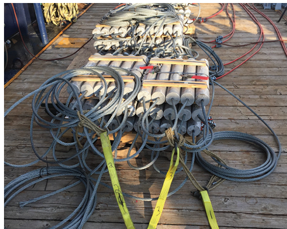
FAR REACHING PROTECTION Each RetroLink™ anode string was 200 feet long with a 25-foot leader.
